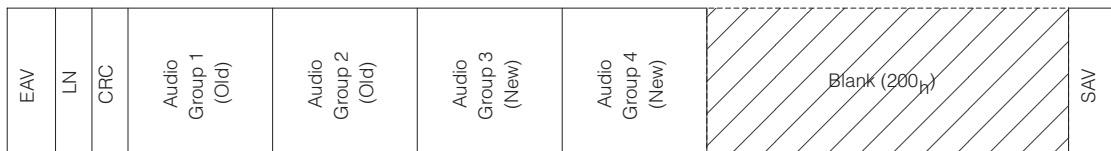
Video Signal after GS1503 Insertion of Audio Groups 3 & 4 (CASCADE = 1)
